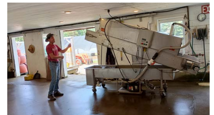
The rinse conveyor cleans and cools individual vegetables
